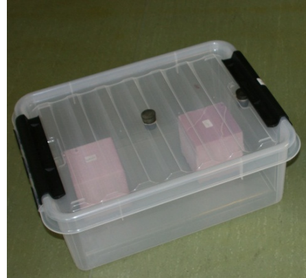
Picture 5: Positioning of insulation blocks in test boxes.
