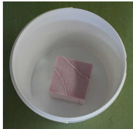
Picture 4: Positioning of insulation blocks in test buckets.
